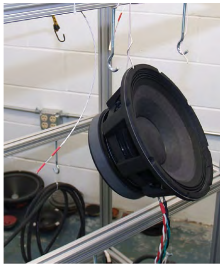
Power testing a high-performance woofer in free air.
