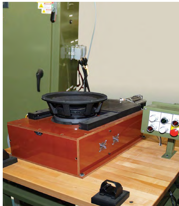
A custom-made high-speed magnetizing system.
