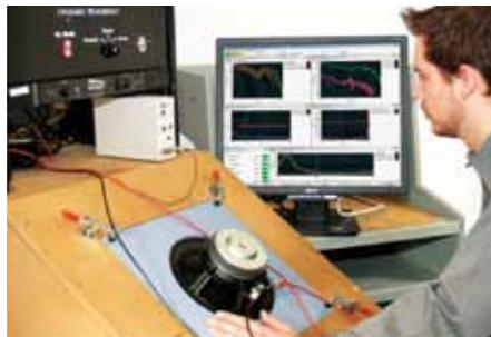
**End-of-Line testing validates customer specified product parameters.**
