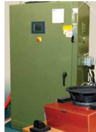
**Massive 3.4 Kilojoule Magnetizer for large neodymium or ferrite magnet structures.**
